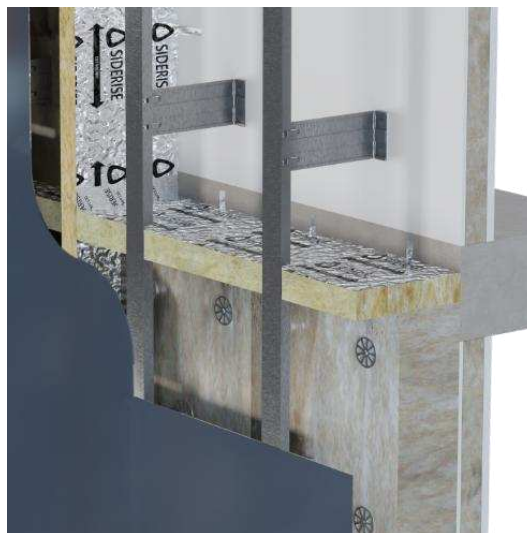
Horizontal cavity barrier in external wall – Image courtesy of Siderise Ltd
