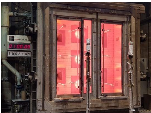
A pair of uninsulated fire doors being tested for fire resistance
